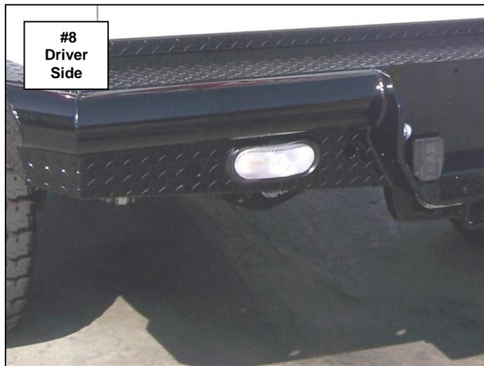
**Step-8** Align the replacement bumper with the vehicle, verify that the tailgate clears when lowered, and tighten all nuts and bolts. If necessary, loosen the nuts and bolts to adjust the bumper. Remember to check and retighten the nuts and bolts periodically.
