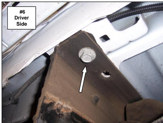
**Step-3** With assistance, lift the replacement bumper up to the frame and position the bumper brackets inside the frame rails. Slide the bumper forward to align the holes and secure each bracket to the frame using (1) 3/8" x 1 1/2" & (2) 1/2" x 1 1/2" hex bolts, flat washers and flange nuts. Leave the nuts and bolts loose for final adjustment. **Picture #7**
