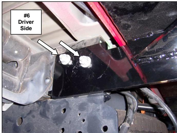
**Step-7** Align the spacer plates with the front bolt plates and slide the spacers between the receiver hitch and frame. **Picture #7**
