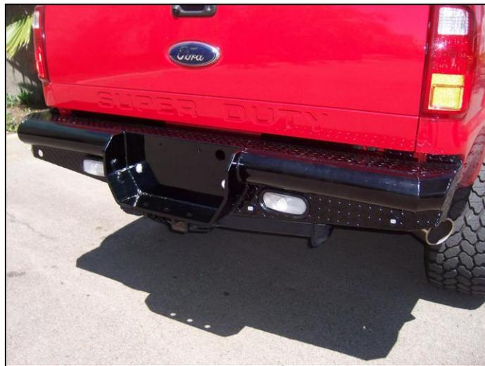
**Step-8** If the vehicle is equipped with back up sensors, Remove the sensors and wiring harness from the factory bumper. Install the sensors in the replacement bumper using the provided rubber grommets then reconnect the factory bumper wiring harness to the sensors and to the vehicle wiring harness.
