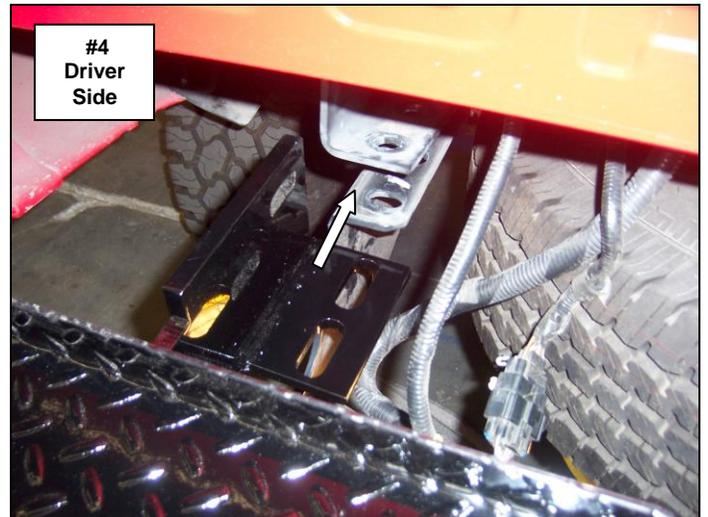
**Step-5** Align the holes and secure the brackets and receiver hitch to the bottom of the frame using the bolt plates and nuts removed in step 3. **Picture #5** Leave the bolts loose for final adjustment.
