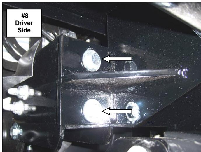
**Step-3** Install the auxiliary brackets by positioning the end with the welded nut inside the frame and the opposite end on top of the bracket welded to the lower tube of the replacement bumper. Align the holes and secure the auxiliary bracket to the frame using (1) 1/2" x 1 1/2" hex bolt and (1) 1/2" flat washer.
