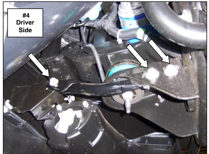
**Step-5** Remove the nut and bolts' securing each of the tow hooks to the frame using an 18mm wrench, socket, and ratchet. **Picture #5**
