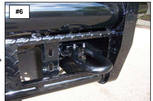
TOW HOOK INSTALLED.
