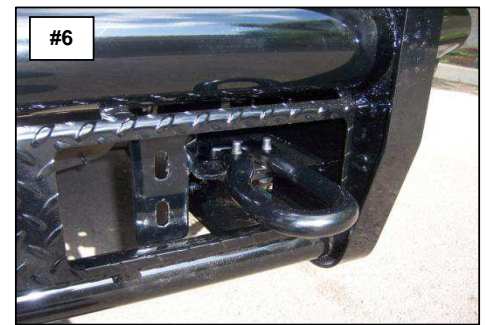
TOW HOOK INSTALLED.
