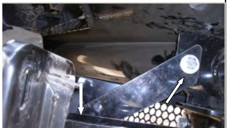
**Step-4** Re-install the hood hook device and the dust cover using the factory fasteners. Install the hood hook auxiliary bracket to the holes in replacement bumper in the end of it, next the grille, using the removed factory fasteners and re-install the hood hook device to this auxiliary bracket as it was in factory bumper.
