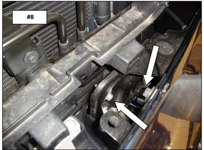
**Step-7** position the driver side upper bracket behind the bumper, align the bracket with the hole in the bumper and bumper frame bracket then reinstall and tighten the bolts, (**Photo 9 & 10**). Repeat the above steps to install the passenger side upper bracket then reinstall the vehicle's grille, radiator cover.
