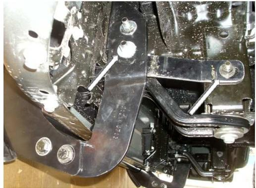
9. Attach the defender with 1/2" x 1 1/2" hex bolts, flat and lock washer and hex nut hand tighten. PHOTO # 7 y 8
