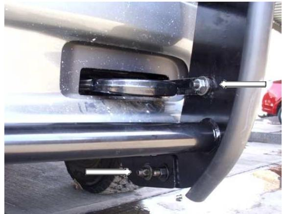
10. Align the defender with the front of the vehicle and tighten all nuts and huts. PHOTO # 9 y 10
