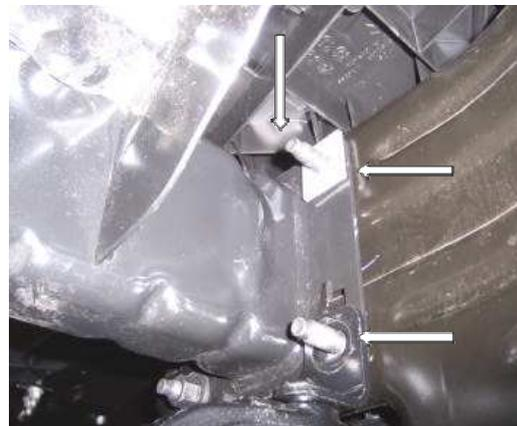
6. position the passenger side frame bracket over the studs and secure the bracket to the frame using the (2) factory nuts. Do not tighten. Photo#3
