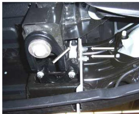
8. To install the auxiliary bracket use the provided template to cut out the bumper's lower cover position the auxiliary bracket through the opening cut out in the lower cover. PHOTO #5 Secure to the tow hook support using a 7/16" x 5" hex bolt, flat and lock washers, and hex nut. Also Attach to the lower bolt of the main bracket. Do not tighten yet repeat the procedure to the opposite side PHOTO #6
